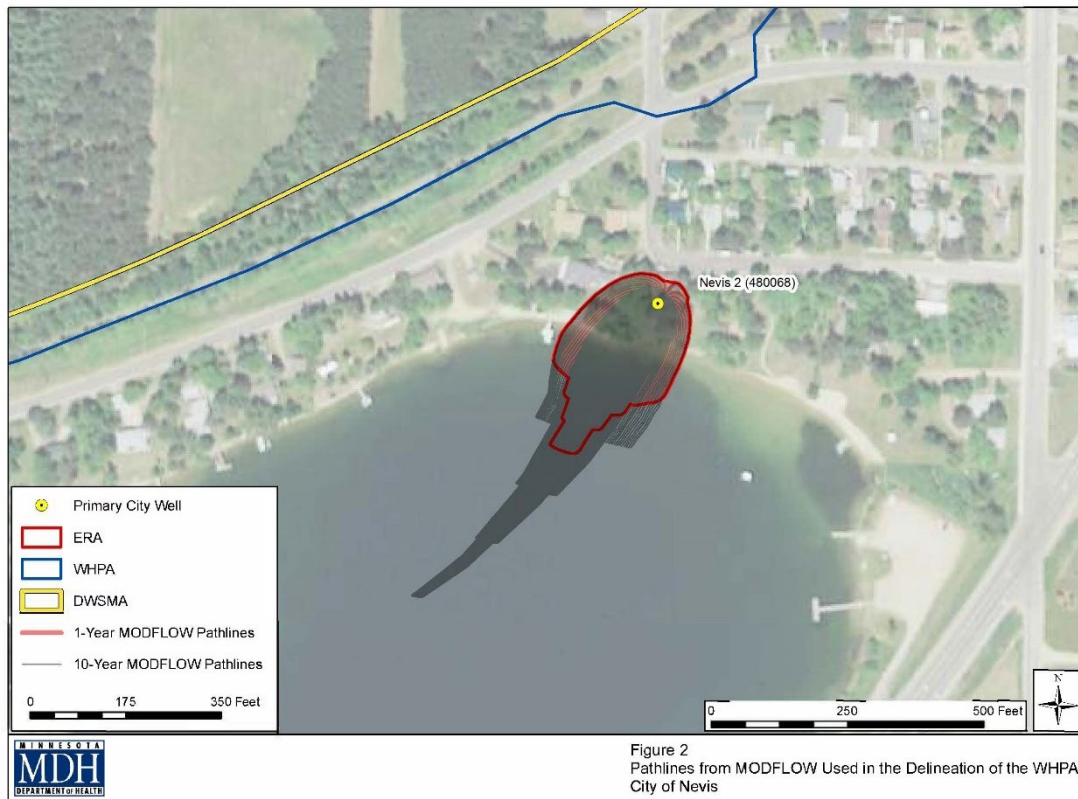
Figure 14. Particle tracks from groundwater flow model, showing capture of lake water within the ERA.
