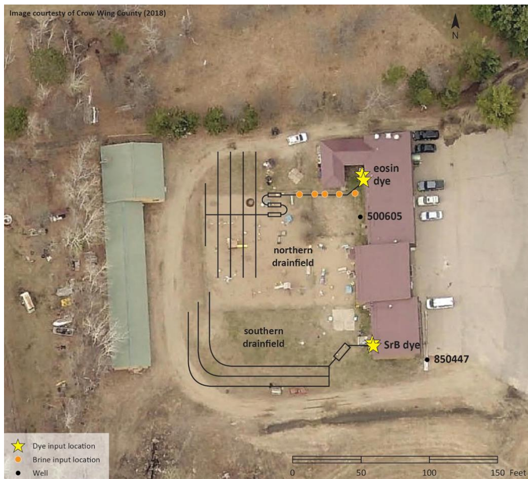
Figure 39. Brine and dye injection locations and associated stormwater conveyance infrastructure. Black dots represent on-site wells. Well 500605 was sampled for this study, while 850447 was used for water level observation. Image courtesy of Crow Wing County.
