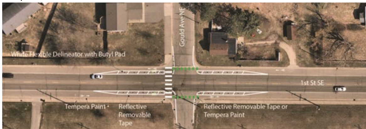
Figure 2: Demonstration Project Design
